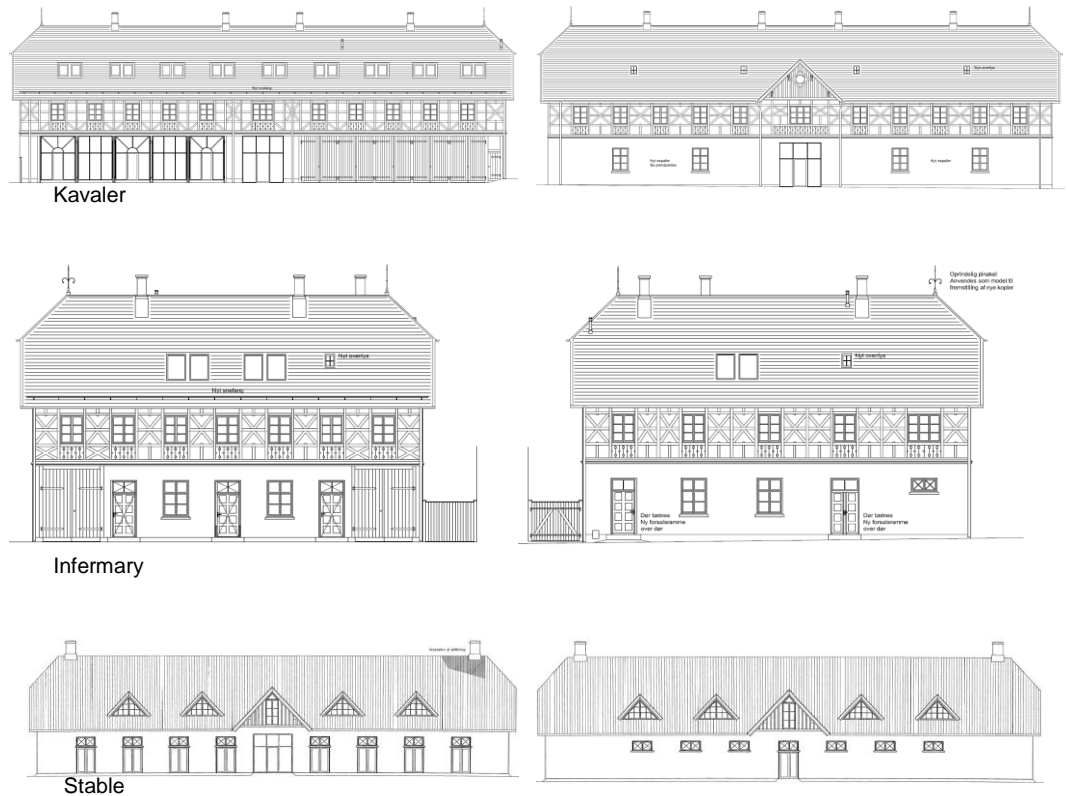
Figure 3: Renovated facades of the 3 buildings – Kavalier (top), Infirmary (middle) and Stable (bottom). Facades to the left are facing the courtyard.
