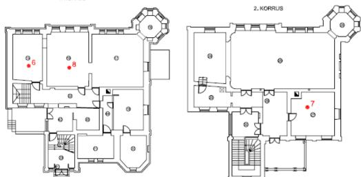
Figure 4 Data loggers location in building Tiigi 11
