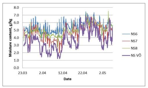
Figure 6 Outside and indoor air moisture content in Tiigi 11 building (spring period)
