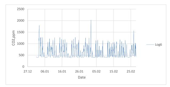
Figure 7 First floor room air carbon dioxide content within cold period
