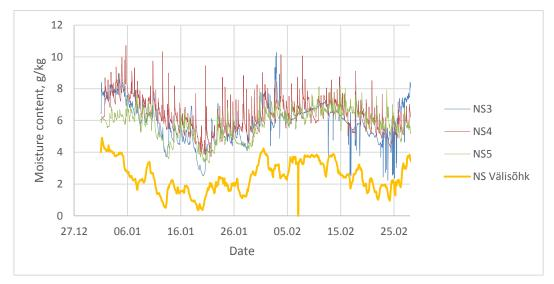
Figure 123 Indoor air moisture content in comparison to outside air moisture content
