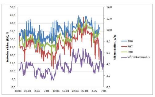
Figure 5 Outside air moisture content and indoor air relative humidity correlation in Tiigi 11 building (spring period)
