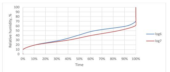
Figure 8 Duration diagram of the room air relative humidity in Tiigi 11 (annual period, working hours only)
