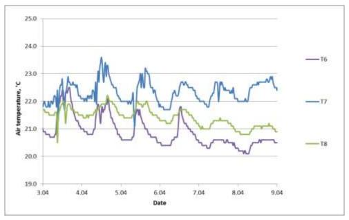
Figure 3 Indoor air temperature in Tiigi 11 building during the week period, when outside air temperature varied -6...6 °C
