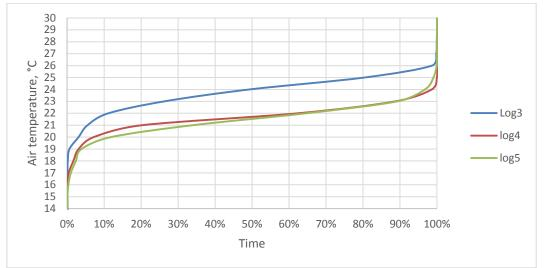
Figure 14 Duration diagram of the room air temperature in Herne 32 (September-May)
