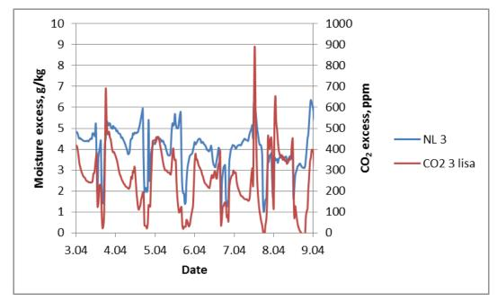
Figure 22 Indoor air moisture excess to CO<sub>2</sub> excess dependency
