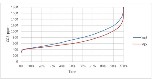
Figure 10 Duration diagram of the room air carbon dioxide content in Tiigi 11 (annual period, working hours only)
