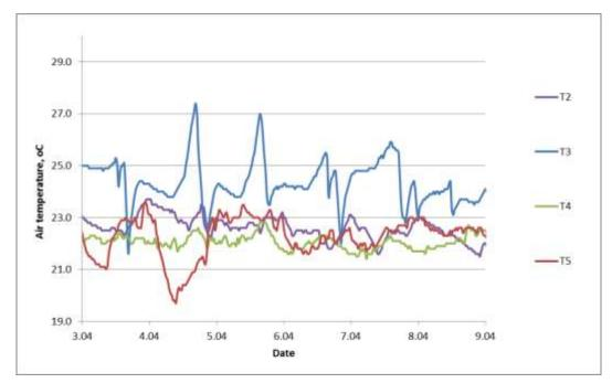
Figure 11 Indoor air temperature in Herne 32 building during the week period, when outside air temperature varied from -6 to 6  $^\circ C$
