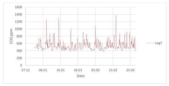
Figure 8 Second floor room air carbon dioxide content within cold period
