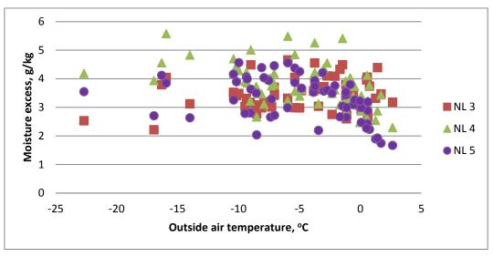
Figure 14 Daily average indoor air moisture excess depending on the outside air temperature
