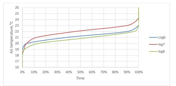
Figure 6 Duration diagram of the room air temperature in Tiigi 11 (September-May, working hours only)
