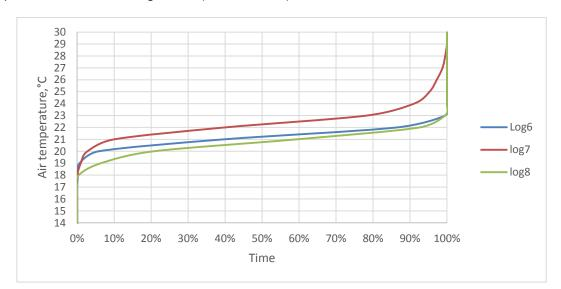
The following duration diagram (Figure 6) displays the measured annual indoor air temperature within working hours (9:00 - 17:00).
