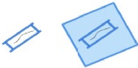
Figure 7. Damaged polyethylene film must be repaired in two layers
