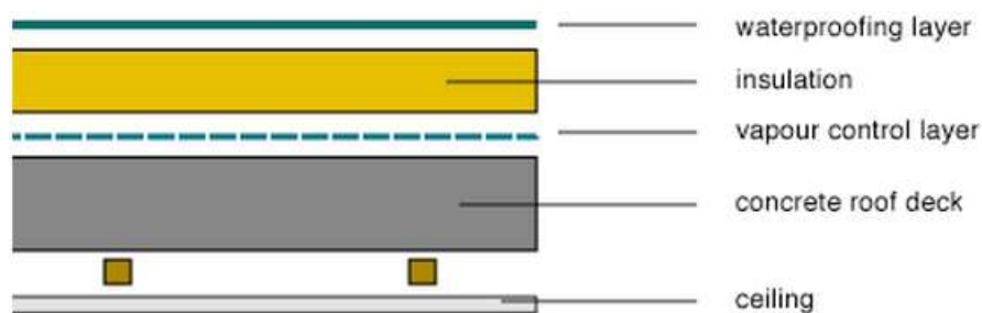
Fig.2.4. Warm roof covering [14]
