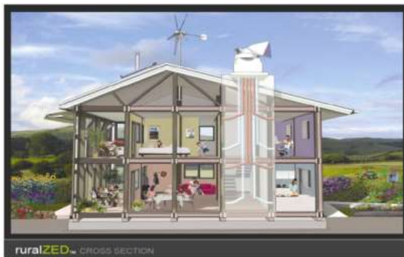
Fig.3.2. Active natural ventilation system [32]
