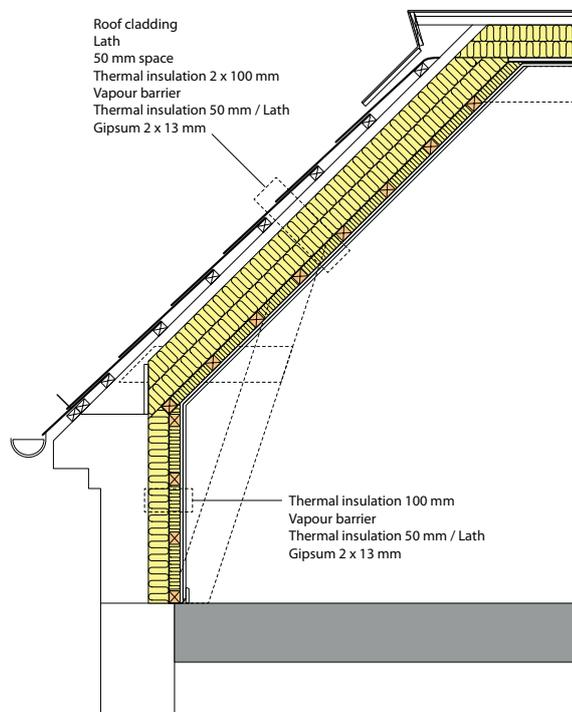
*Vertical section of the roof above the apartment in the former attic room.*
